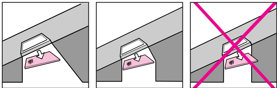
**English:** Decide on the design of the light shaft. Optimum light distribution and increased air circulation are obtained with flared/expanded light shafts.
